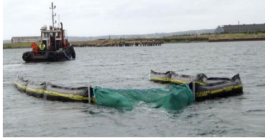
The Debris Trawl/River Sweep (alias the Scan Trawl) (source: DESMI)
