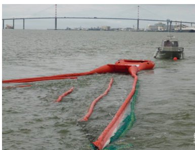
View of the Lamor MOS 15 with its deflectors concentrating the pollution towards the recovery channel and collector pool (source: Cedre)
