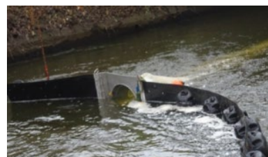
Above: The Trash Trap (top) and Trash Tube, here coupled with GlobeBoom
