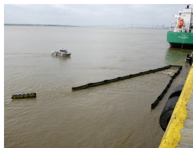
Positioning of the Speed Sweep in static configuration using the Ro-Kite (source: Cedre)
