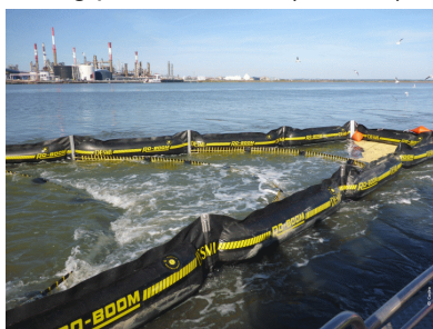
Attenuation of the surface current by successive Kevlar screens integrated in the DESMI Speed Sweep (source: Cedre)
