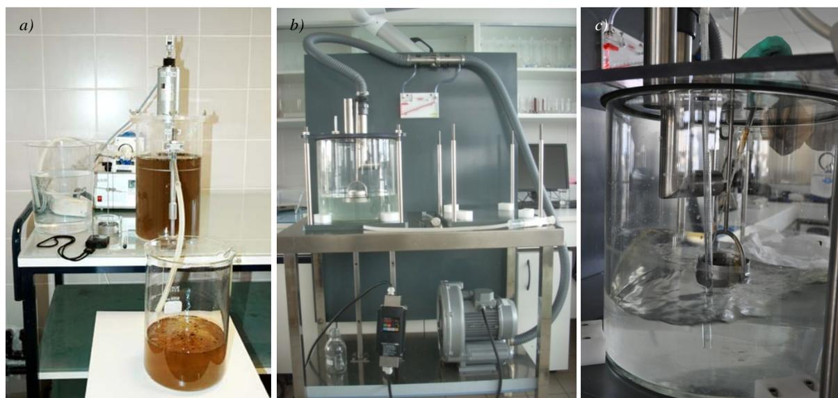
**Figure 1** Experimental set-up used for the a) IFP and b), c) MNS tests.
