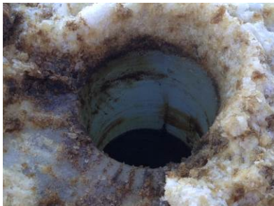
Visible presence of oil: hole drilled in the ice (left); oil surfacing through cracks in the ice (5 km downstream of the slots) (right) (source: US EPA)
