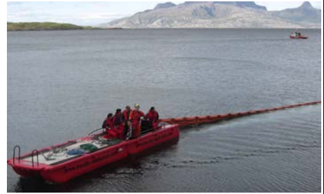
Deploying booms from the double hulled Seahunter with a 25-hp engine (LSH 25 SC) (Source: Lamor)
