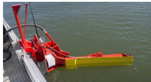
The MiniBagger sweeping arm (Source: SeaHow)
