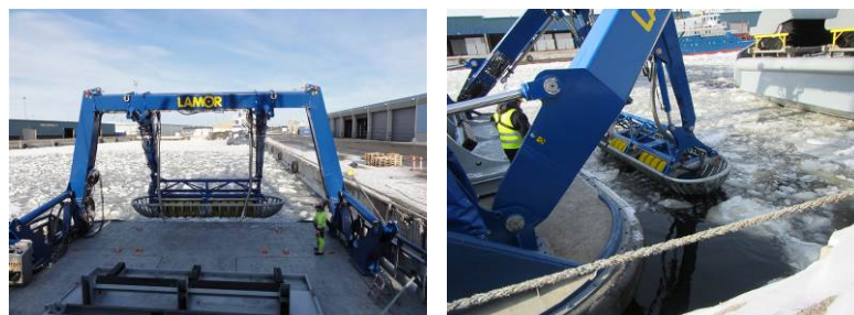
The Sternmax fitted to the stern of a spill response vessel (Source: Lamor)
