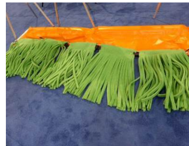
IOSC 2014: OPFLEX sorbent Cube Boom (left) and Eelgrass (right, here used with sections of fence boom) (Source: Cedre)
