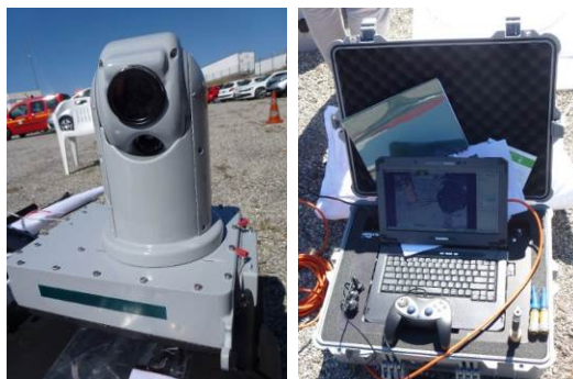
View of the turret with IR and video cameras (left) and of the compact command panel (right) (Source: Cedre)
