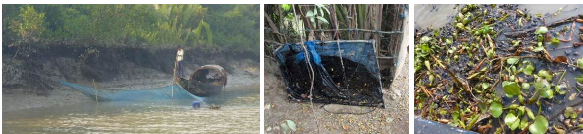
Fishing net at the edge of the bank (left); Net attached to a frame (centre); Trapping oil using water hyacinths (right) (Source: Cedre)
