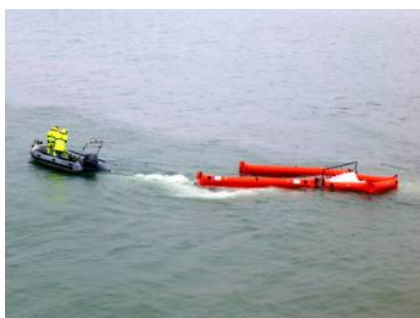
Dynamic recovery by trawling in the Brest roadstead (Source: Cedre)
