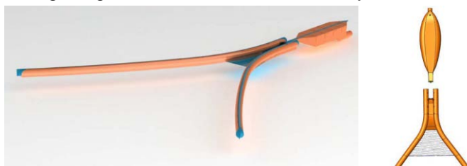
Diagram of the Oil Trawl system (Source: www.norlense.no )
