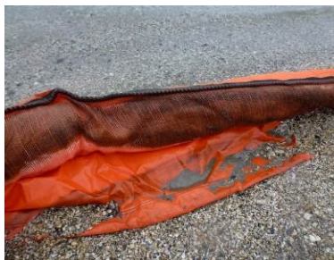
Western section of Jai beach: preliminary mixing test (low pressure lances) on oiled sediment: recovery, using sorbent booms, of the oil trapped in the sediment and remobilised by water jets (Source: Cedre)
