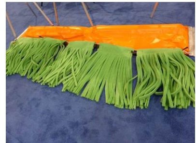
IOSC 2014: OPFLEX sorbent Cube Boom (left) and Eelgrass (right, here used with sections of fence boom) (Source: Cedre)
