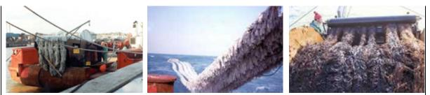
Drawing upon the skills of the SMEs involved in this project, the main amendment to the system resides in the type and design of the oleophilic materials used. The 5 pairs of strands of polypropylene fibres, 75 cm wide, have been replaced with 4 multilayer bands designed to promote the recovery and retrieval of heavy oil, while also being efficient on light oils.
