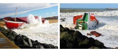
airlifted to safety at around 06/02/2014: Bow section of the Luno on Cavaliers beach (left) and bridge grounded at the end of the Cavaliers breakwater after breaking away from the stern section (right). No pollution was visible on the water or the foreshore (Source: Cedre)
