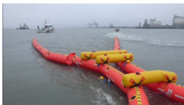
Dynamic mode : Left: pair towing (by a 19 m buoy tender provided by the Saint Nazaire subdivision of Phares et Balises + a small 7.5 m cruiser belonging to FOST); Right: towing by a single vessel, with deployment by an ORC BoomVane (Source: Cedre)
