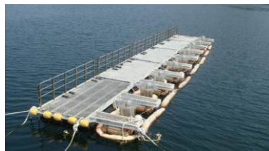
View of the mesocosms developed by KIOST: polyethylene cylinders (left); floating pontoon comprising the 9 experimental cylinders (above). (Source: Joo et al., 2013)
