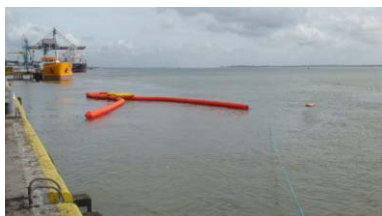
Static mode : the Current Buster 4 moored to a fixed point, deployed using an ORC BoomVane.
