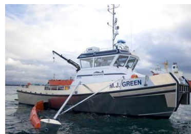
Outrigger and sweep boom of the Rozema 47 (Source: Elastec)
