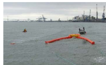
Dynamic mode : Left: pair towing (by a 19 m buoy tender provided by the Saint Nazaire subdivision of Phares et Balises + a small 7.5 m cruiser belonging to FOST); Right: towing by a single vessel, with deployment by an ORC BoomVane (Source: Cedre)
