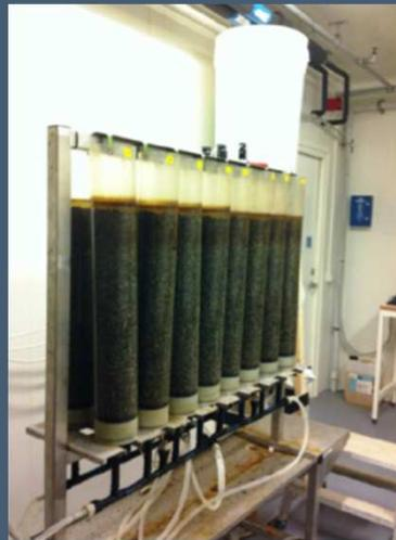
*Sintef column system including a water reservoir*
