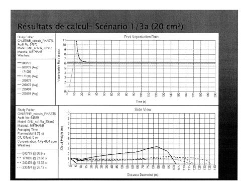
Figure 5Phast Simulation Describing the Extension of a Flammable Zone of<br/>an LNG Tanker with a 20-cm² Hole (Different lines are drawn<br/>depending on the type of atmospheric conditions (See Table 3).<br/>Source: Ineris
