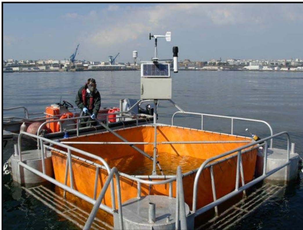
Figure 5 : On site experimental procedure: operator on the boat is pumping samples, PID at the right corner of the floating cell and the meteorological station.
