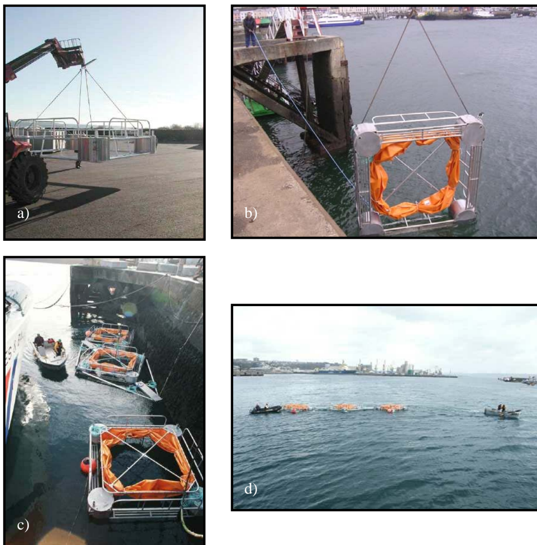
Figure 2: a) The lift of the home-made waterborne frameworks, b) The hanging thanks to a crane-truck c) The launch of the floating cells and d) The tow until the experimental zone with a ship and a rubber dinghy.
