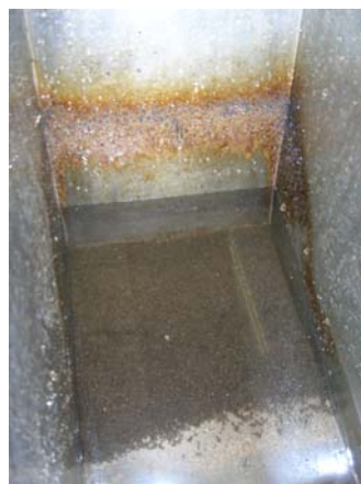
Figure 2. Oil on the walls of a tank after one hour of agitation.
