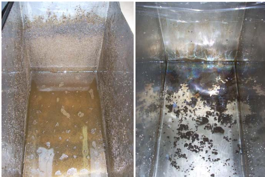
Figure 7. Picture of tanks after one hour of agitation for a sediment polluted with heavy fuel oil at a concentration of 50 mg/g (left) and 110 mg/g (right).
