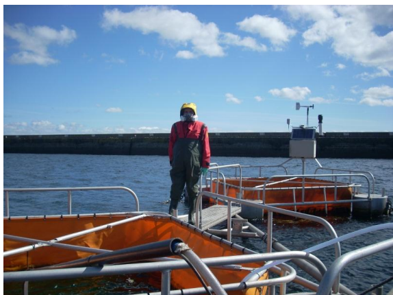
Figure 4: Field trials in floating cells in the Bay of Brest. Source: Cedre
