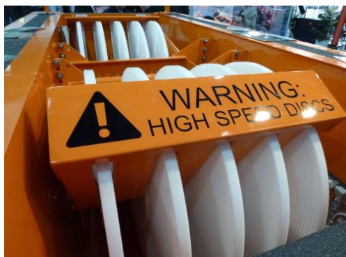
Two series of discs on the X150 skimmer (Source: Cedre)
