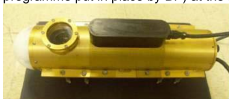
The Oscar prototype, sensor for submerged or sunken oil (Source: EIC Laboratories)
