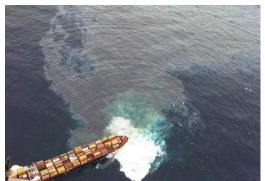
6th October: leak of IFO 380 at sea from a cracked bunker tank (Source: MNZ)
