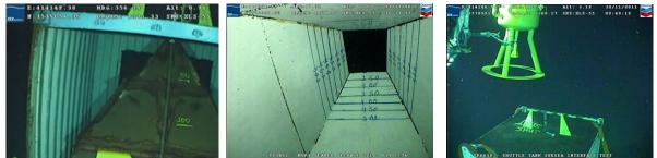
Left: Inside of the steel containment device sitting on top of a seepage point, containing a funnel structure; Middle: View of droplets rising by gravity inside the funnel system of the containment device; **Right**: Placing the shuttle tank on the steel containment device (Source: Chevron)
