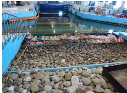
Man-made beach (pebbles) within MERTI's facilities (source: Cedre)
