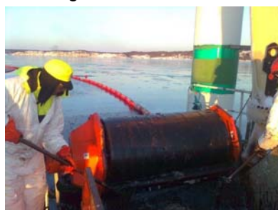
Sandvik industrial steel belt oil skimmer (source: Kystverket)
