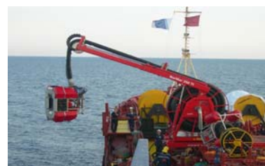
NorMar 250 TI skimmer on board the Aktea (source: EMSA)
