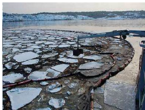
Recovery using a grab (source: Kystverket)
