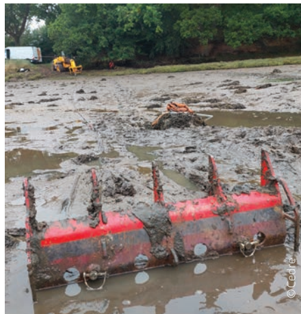
▲ Claw anchor positioned in muddy substrate prior to trial
