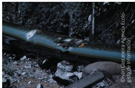
^ View of the breach in the pipeline (left); Soil and vegetation in the ravine sprayed by the pressurised oil spurting from the pipeline (right)
