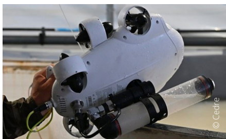
▲ FIFISH V-EVO underwater drone with its sampling syringe (500 mL)
