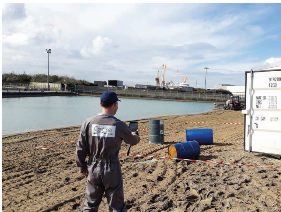
▲ Measuring the temperature increase in chemicals using a thermal camera
