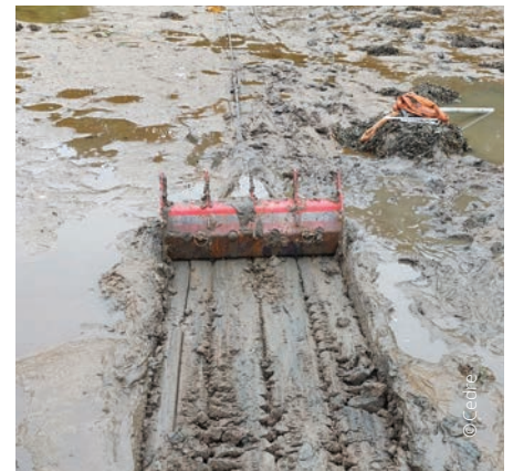
▲ Claw anchor after trial in muddy substrate
