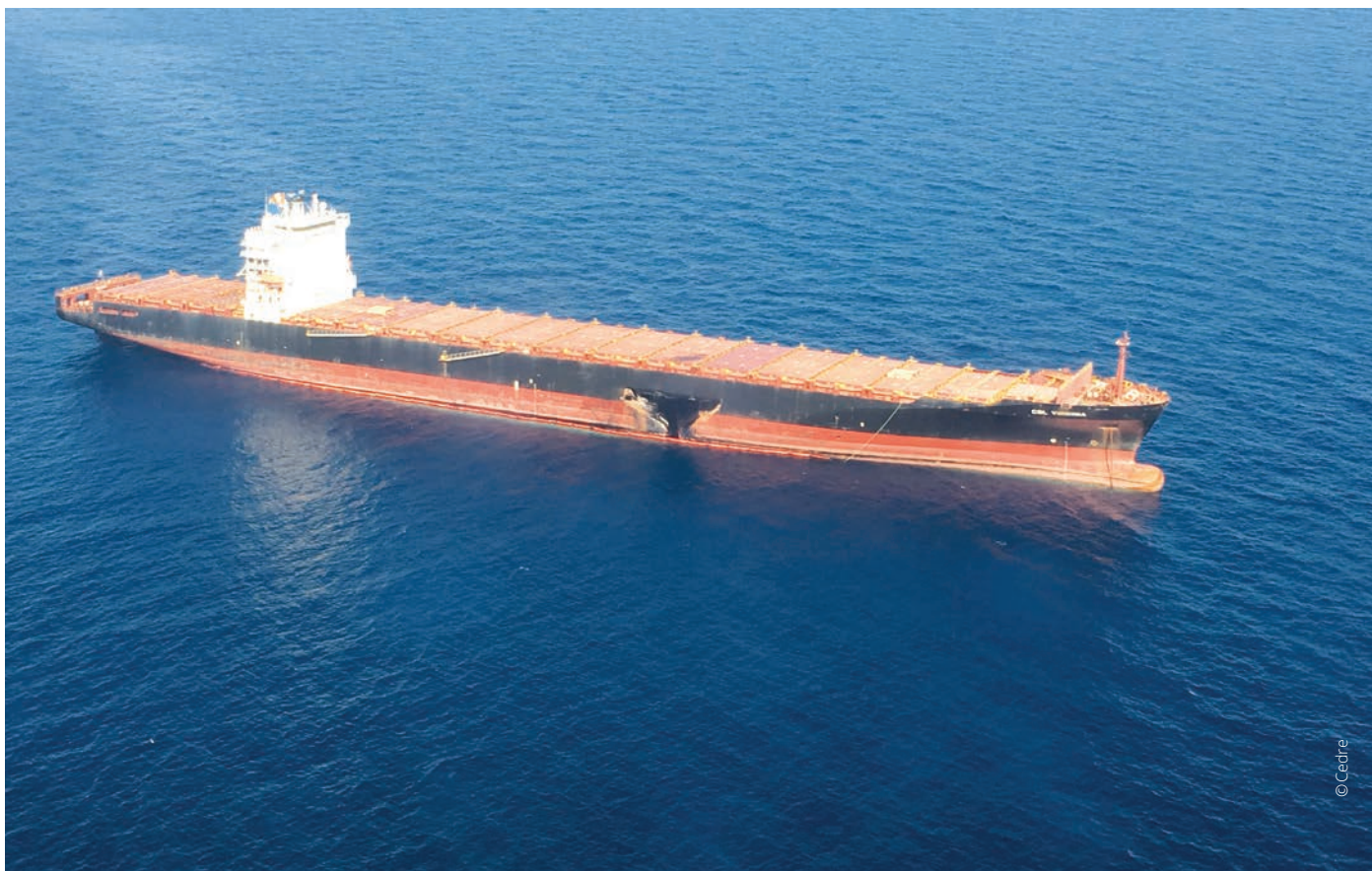
△ Overflight above the container ship CSL Virginia and view of the breach in the ship's hull (France, October 2018)
