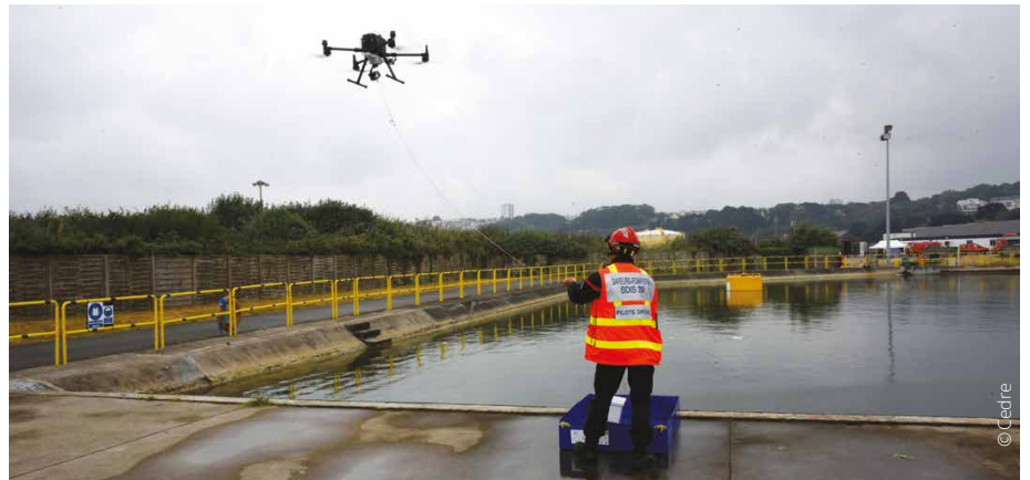
^ Testing UAVs and sensors above Cedre's test tanks as part of the IRA-MAR project
