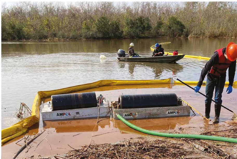
^ Recovering the thickest accumulations of diesel along the banks using oleophilic drum skimmers (Source: Louisiana Department of Environmental Quality)
