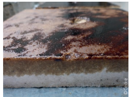
▲ Penetration of a VLSFO in a slab of granite
