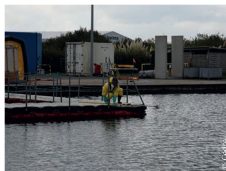
^ Chemical spill in Cedre's outdoor test tank, and detection by the Belgian Civil Protection with a detector using infrared spectrometry
