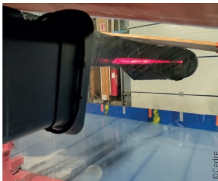
▲ Measuring droplet size in a spray plume using a laser diffraction system
