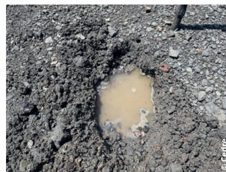
▲ Subsurface inspections to check the level of cleanliness of a sediment foreshore (stones on sandy mud) treated by flushing (with low pressure hoses) to extract the infiltrated oil
