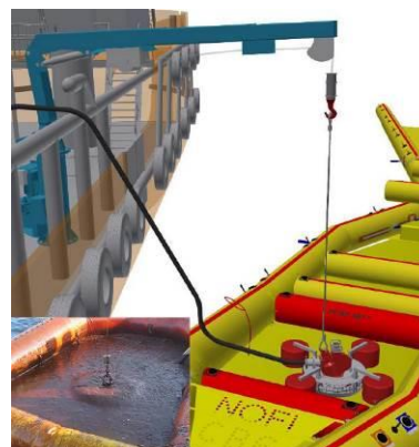
Modelling and photograph of the deployment of the NorMar 4 Discharge System (source: AllMaritim)
