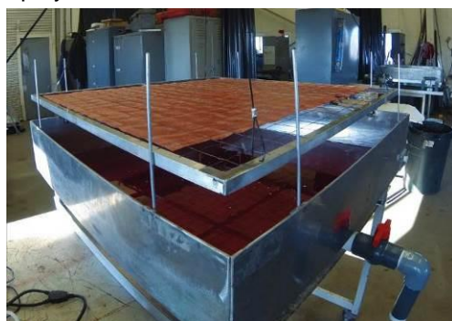
Prototype structure/mount for sorbents (pads, mats) for standardised tests (source: Ohmsett/BSEE)
