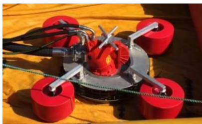
DESMI DOP-200 DUAL pump on aluminium frame with removable floats (source: AllMaritim)
