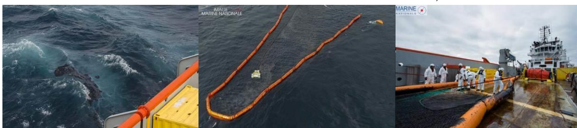
Left: Appearance of the emulsified fuel oil, fragmented into viscous clusters (14.03.2019); Centre: offshore containment operations on patches of fuel oil using booms (here deployed using a boom vane), and skimming operations using a Lamor offshore skimmer (weir + brush module), operated from the Argonaute via a reel-mounted umbilical (19.03.2019); Right: Hauling a Thomsea surface trawl net, used to recover scattered clusters of viscous fuel oil, onto the deck of the Argonaute (source: French Navy)
