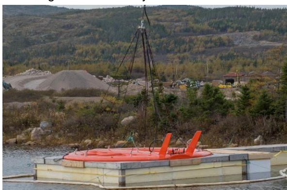
Left: view of the reinforced NMR antenna prototype (Ø = 6 m) being tested in Newfoundland (Canada) in 2016; Right: deployment by helicopter (source: Palandro et al., IOOSC 2017)
