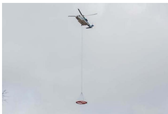
Left: view of the reinforced NMR antenna prototype (Ø = 6 m) being tested in Newfoundland (Canada) in 2016; Right: deployment by helicopter (source: Palandro et al., IOOSC 2017)
