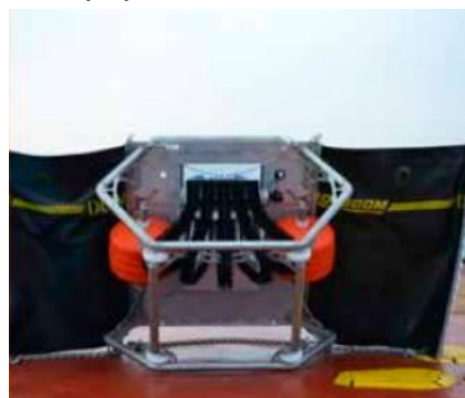
View of the front panel (i.e. “internal” view) of the Octopus In-Line skimmer (source: DESMI)
