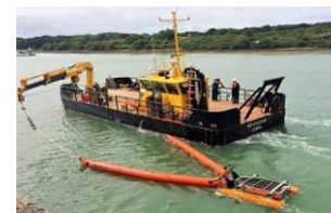
Maxi Fasflo deployed in dynamic mode (source: Vikoma)
