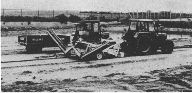
Figure 4. Field test of ROLBA kit on CEDRE's experimental beach
