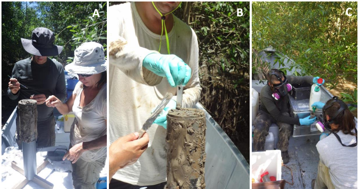
Figure 4 (A) Sampling of the sediments for the microbial analyses. (B) Sampling of the sediments for the analysis of the meiofauna. (C) Fixation with formaldehyde (4% final concentration) of the sediment samples for the macrofauna and meiofauna analyses.
