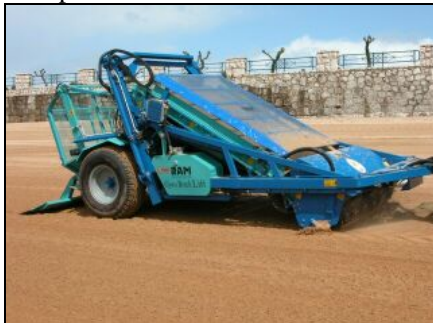
Ram Gyro Beach Lift (source : Cedre)
