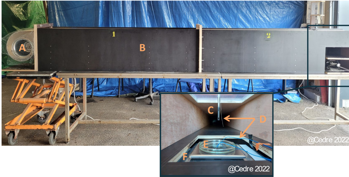
Figure 2. Panoramic view of the wind tunnel with a close-up image of the petri dish and the operating sensors inside the gallery: A) fan; B) tunnel; C) anemometer; D) thermocouples; E) petri-dish and F) weighing scale.
