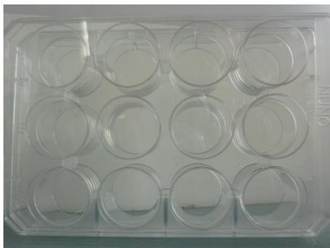
Figure 4: Multiwell plate used for toxicity testing on *Artemia* larvae and cysts.
