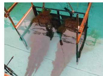
Mesoscale testing in the Ohmsett tanks (Source: BSEE)
