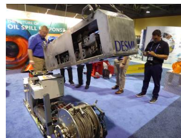
Prototype of the DESMI igniter (suspended)/herder application (on floor) system (Source: Cedre)
