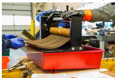
Oil extraction tests using the wringer system (Source: Argonne National Laboratory)
