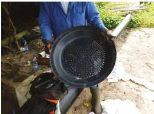
A perforated bin lid made to recover sections of root
