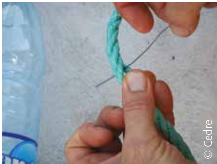
Threading the wire between the strands of the rope before binding the bottle to the rope
