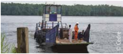
Waste pooling barge complete with suitable containers
