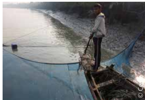
Traditional shrimp boat used in a stationary position alongside the bank to recover clumps of oil and oiled aquatic plants
