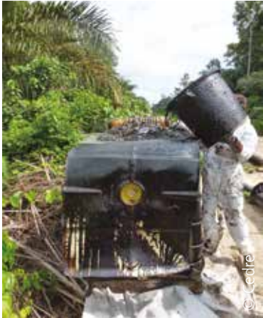
Unloading vegetation onto the screen using a bin and draining it
