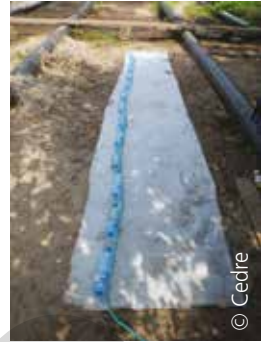
Preparing the necessary materials, laying the strip of geotextile on the ground, laying the rope then the bottles
