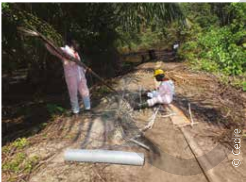
Laying out the casing on the ground and filling with fibres
