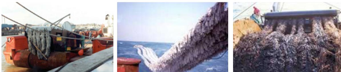
Drawing upon the skills of the SMEs involved in this project, the main amendment to the system resides in the type and design of the oleophilic materials used. The 5 pairs of strands of polypropylene fibres, 75 cm wide, have been replaced with 4 multilayer bands designed to promote the recovery and retrieval of heavy oil, while also being efficient on light oils.
