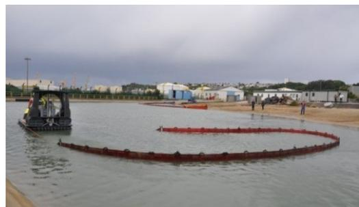
Cedre's water basin and man-made beach: towing a boom in a trawling configuration (source: Cedre)
