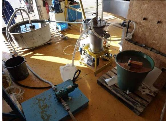
Testing the Turbylec, at Cedre, together with a DESMI Terrapin skimmer and a Börger AL25 pump (Source: Cedre)
