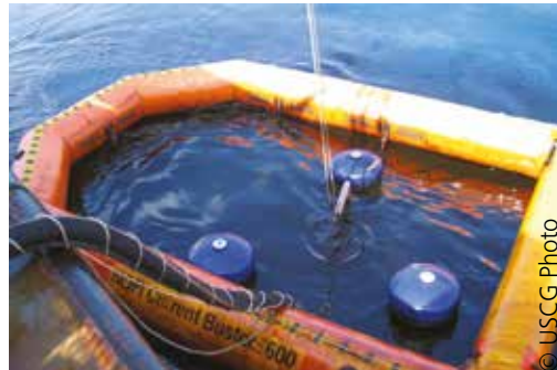
Skimming oil while using a boom to concentrate the oil, Gulf of Mexico spill (2010)
