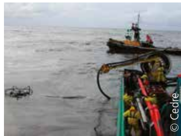
Optimising the use of a skimmer by deploying a containment boom
