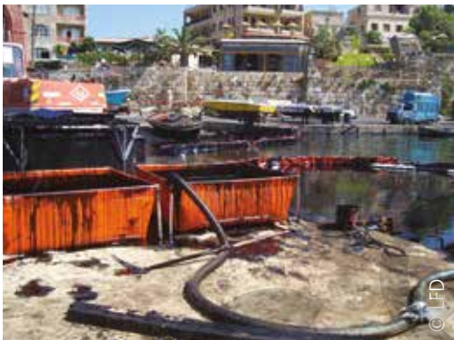
Flexible framed storage tanks
