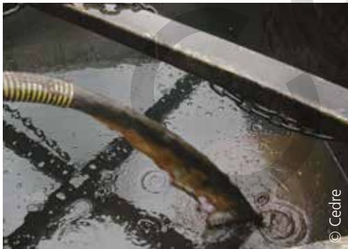
Transferring a fluid oil and water mixture to a storage tank
