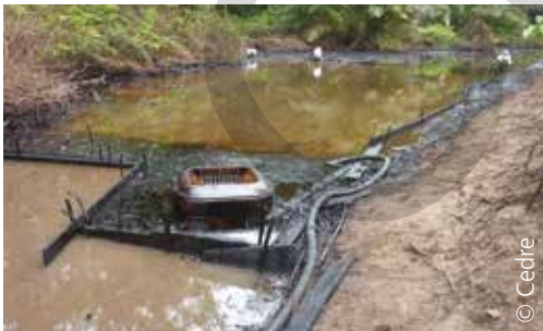
Disc skimmer deployed in the presence of floating debris
