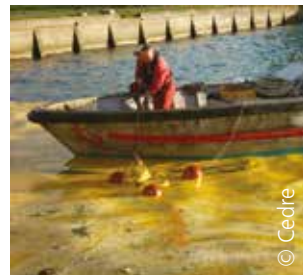
Floating solid waste can clog up skimmers and prevent them from operating correctly
