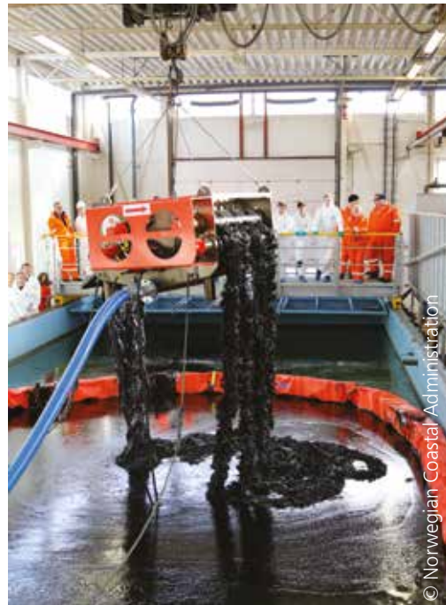
Skimmer trials at the NCA test facility in Horten
