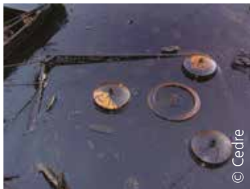
Floating solid waste can clog up skimmers and prevent them from operating correctly
