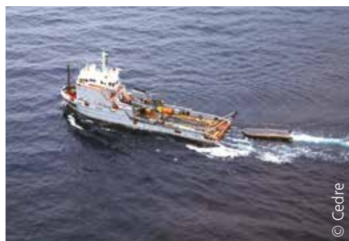
Storage bladder being towed
