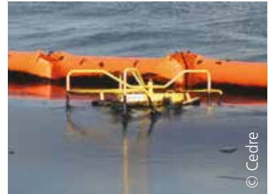
Optimising the use of a skimmer by deploying a containment boom
