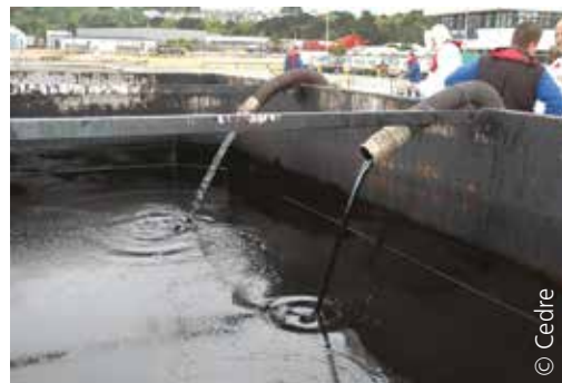
Mixture containing a large proportion of oil recovered by an oleophilic skimmer
