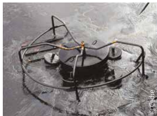
Recovering viscous heavy fuel oil
