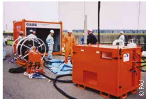
Hydraulic power pack
