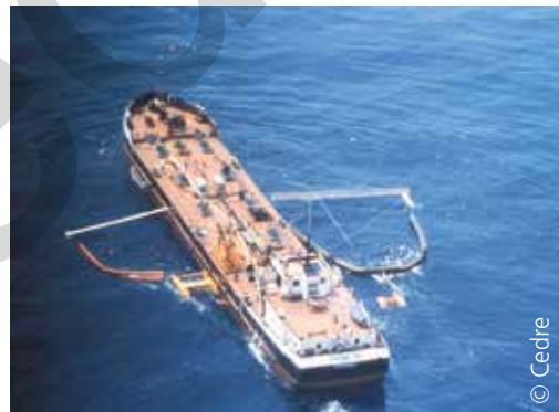
Coastal tanker pre-fitted to deploy skimmers alongside it
