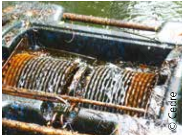
Low recovery efficiency due to excessive brush rotation speed
