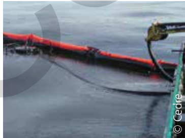
Optimising the use of a skimmer by deploying a containment boom
