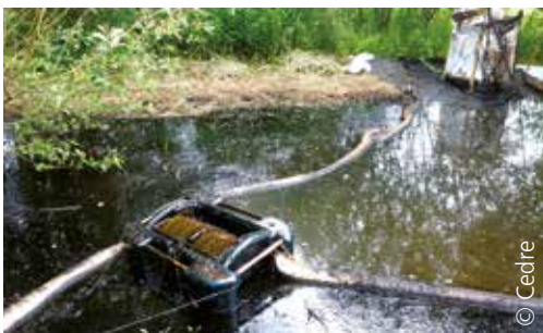
Brush skimmer deployed in the presence of floating debris
