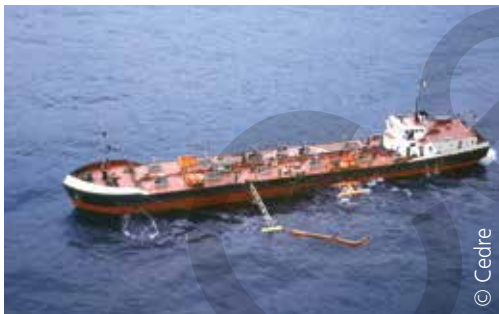
Coastal oil tanker converted into a recovery vessel
