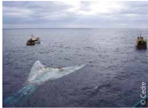
A spill response trawl system being deployed by fishing boats
