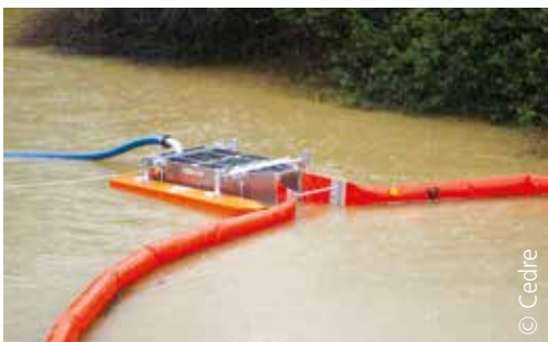
Dynamic recovery using a system composed of a skimmer and sweeping booms
