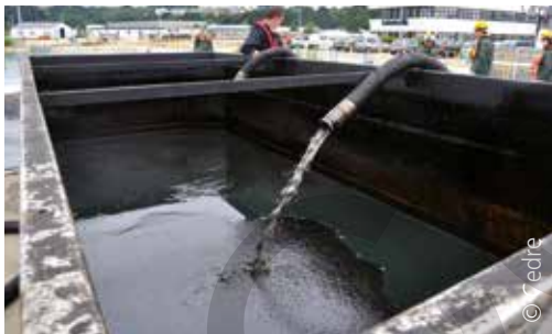
Mixture of oil and water collected by a mechanical skimmer
