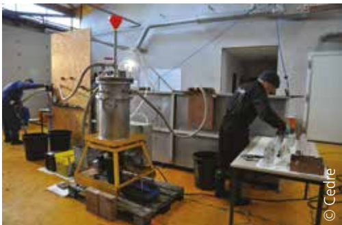
Compact separator test
