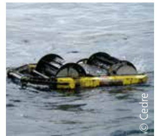
Optimising the use of a skimmer by deploying a containment boom
