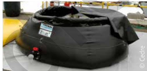
Flexible storage tank fitted with a valve to drain off water after settling
