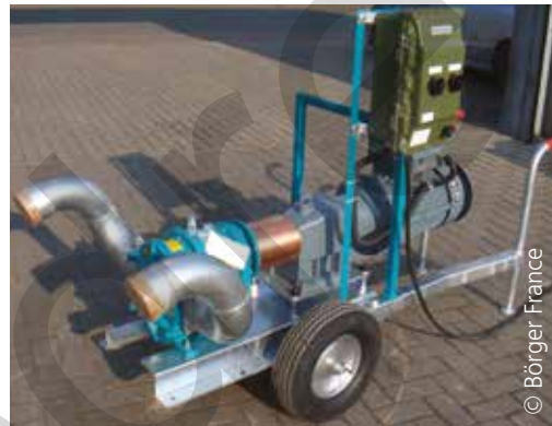
Trolley-mounted ATEX lobe pump with electric motor
