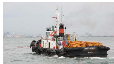
Spraying dispersants by boat (spray arms) (Source: ITOPF)
