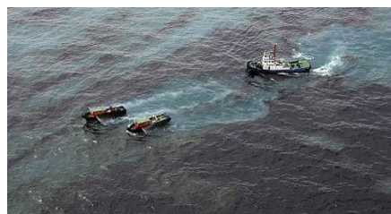
Spraying dispersants using spray arms and fire hoses (Source: Royal Thai Navy)
