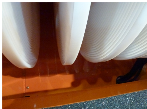
Close-up of the grooved surface of the Elastec X150 skimmer's oleophilic discs (Source: Cedre)
