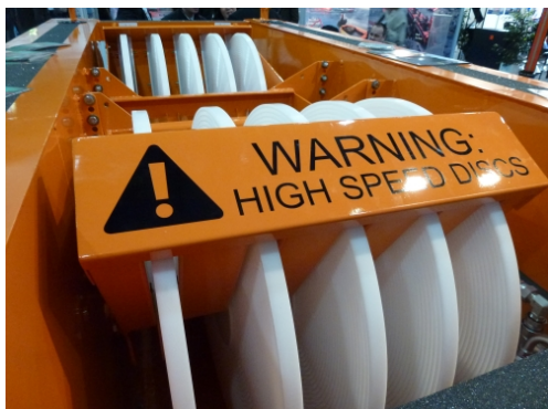
View of the X150 skimmer's two rows of discs (Source: Cedre)
