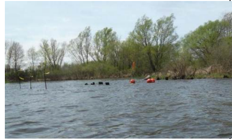
Sediment traps, indicated by buoys on a selected section of the Kalamazoo River
