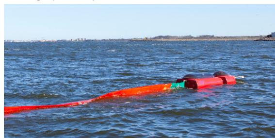
*View of the ASV towing a permanent fence boom
