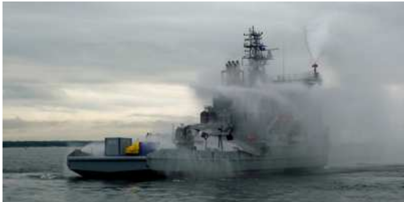
Finnish supply vessel Louhi. This multipurpose vessel built in 2011 is specialised in response to chemical and oil pollution. Here, activation of spraying system for response to chemical pollution and gas cloud - © Cedre
