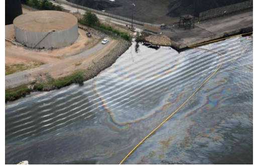
Containing the fuel oil on the water in front of the spill point using floating and sorbent booms (Source: USCG)
