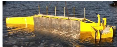
12 m rigid sweeping arm + pump (source: Hebo Maritiemservice)
