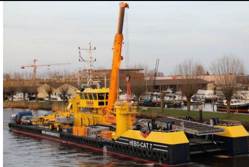
View of the spill response vessel Hebo-Cat 7 (source: Hebo Maritiemservice)
