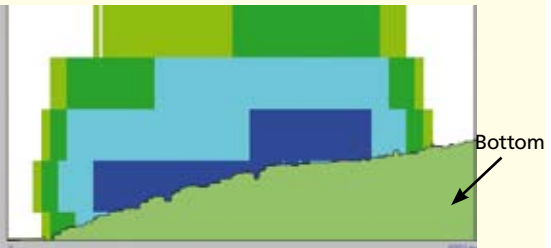
Figure 46: cross-section of dissolved part after 28 h at flood tide
