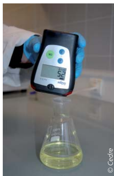
Measuring vapours using an explosimeter.
