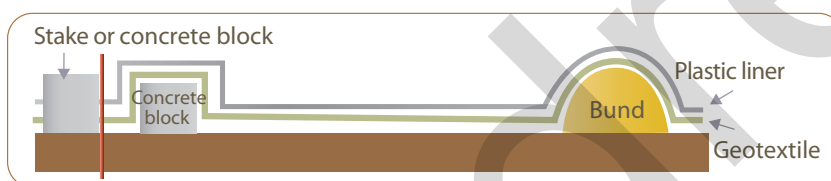
Figure 10: Diagram of a watertight platform for bulk waste (cross-sectional view)
