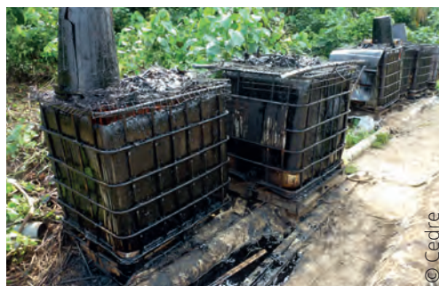
Custom-made drying/draining system: plant debris placed on a grid over an IBC
