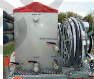
Mobile settling tank that can be set up on site
