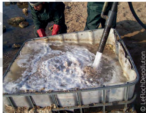
Custom-made sediment/oil separation system using the flushing technique
