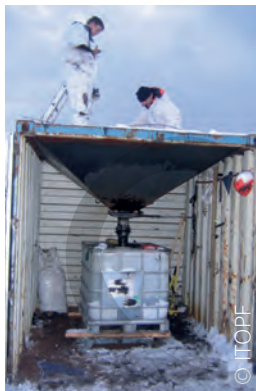
Improvised separation system: screened funnel and separation of oil and litter
