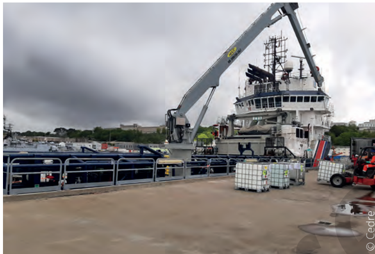
Appropriate lifting equipment for the weight to be lifted: forklift to transport an IBC
