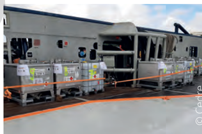
Organised temporary storage of chemicals onboard a vessel
