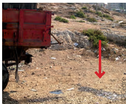
Oil leakage from a non-watertight truck
