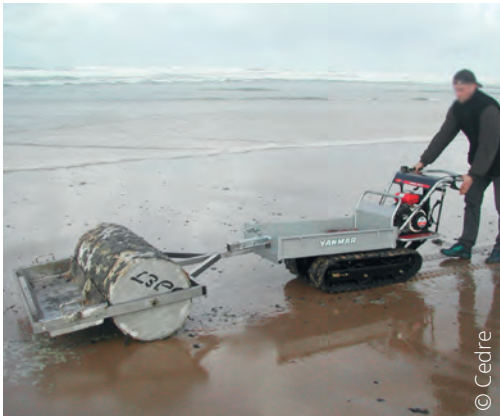
Collection by adhesion of oil to an oleophilic roller
