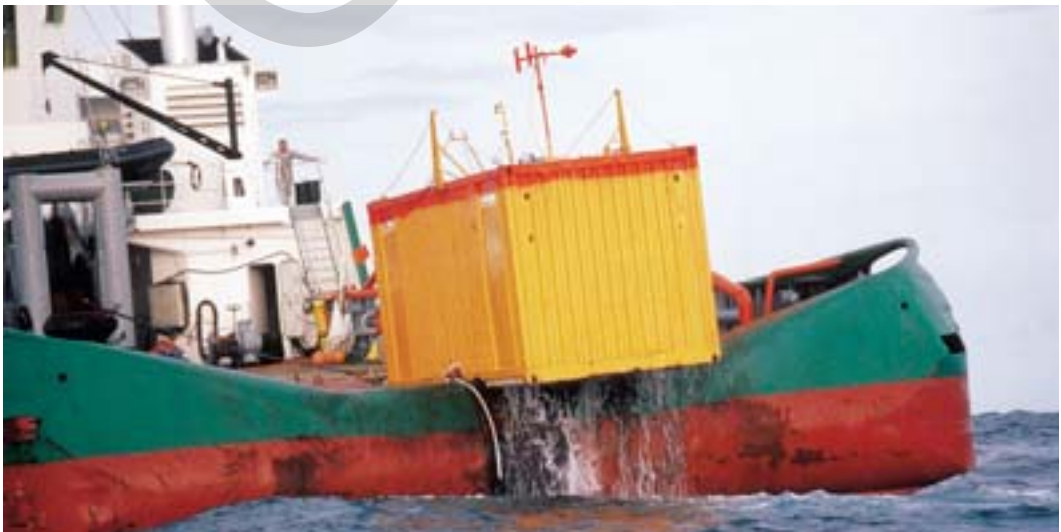
20-foot container fitted with instruments hoisted on board a supply ship (photo Cedre).
