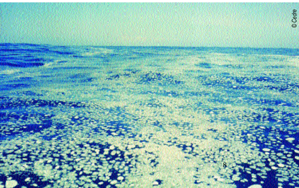
Solidified vegetable oil slick (RAPSODI II experiment)
