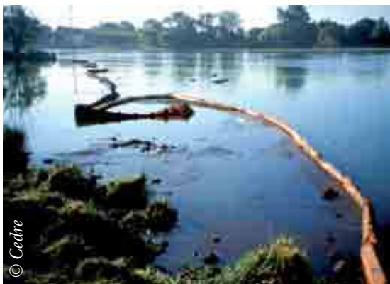
Shallow waters cause the boom to plane; furthermore, the pollutant is distributed throughout the water column
