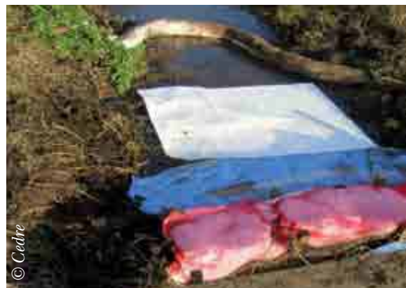
Sorbent boom and pads.
