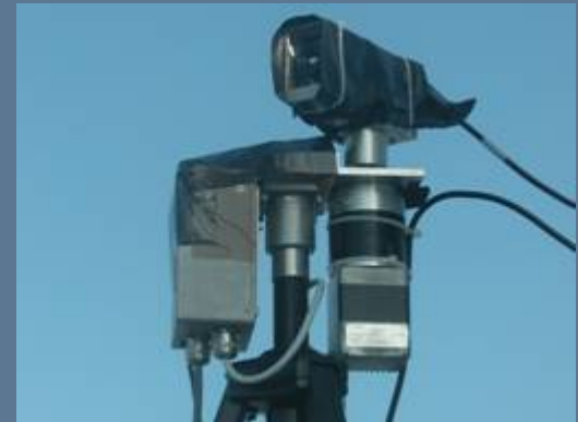
DEPOL 07: the thermal infrared camera of project DETHERPOLMAR – Source Cedre
