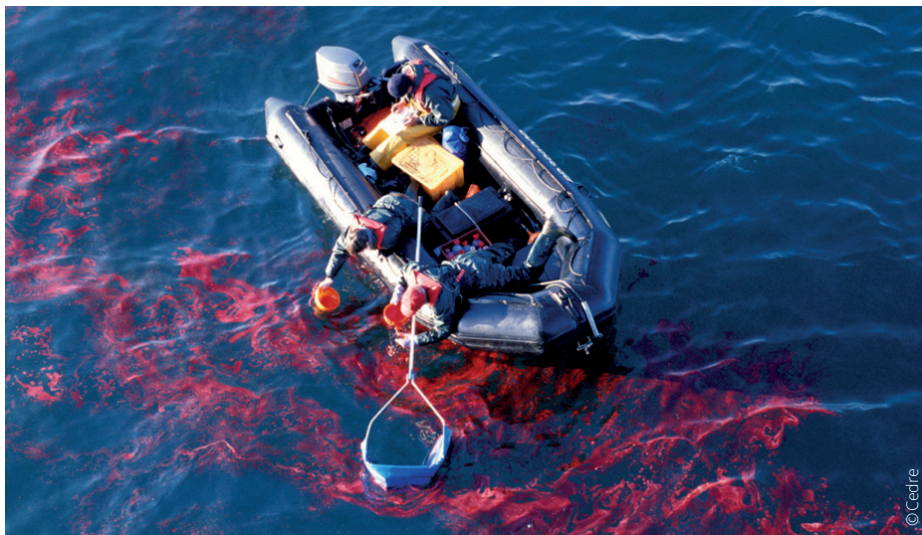
▲ Sampling vegetable oil from a semi-rigid boat during the RAPSODI offshore experimentation off Penmarc'h, Finistère
