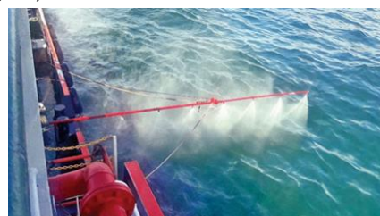
Spraying dispersants from a tug using spray arms (source: Ceylon Petroleum Corporation)
