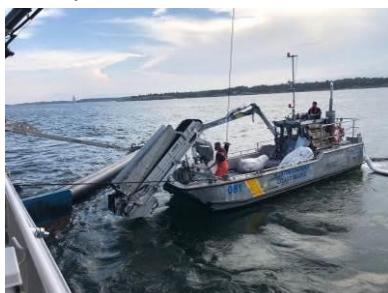
Recovery of floating fuel oil spill from the Makassar Highway in inshore waters: launching an oleophilic skimmer with linear brushes (Lamor Bow Collector) from a recovery barge (left); transfer of the viscous fuel oil stored in the barge's tanks (right) (source: Kustbevakningen)
