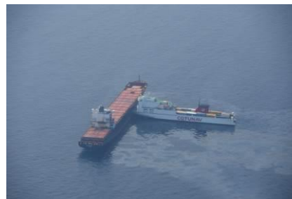
The ro-ro vessel Ulysse lodged in the starboard bow of the container ship CSL Virginia, and leak of bunker fuel from the latter (source: French Navy)
