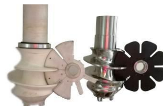
View of the screw and the geared sealing disc of the final version of the SEDOSR Pump One (source: SEDOSR)
