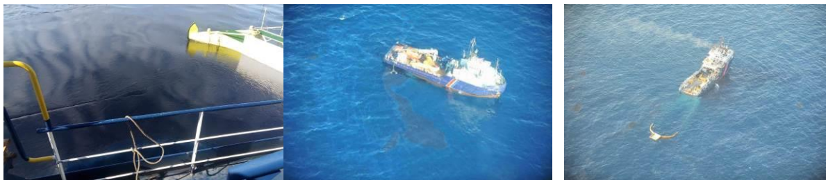
Various recovery methods employed (examples, from left to right): containing a floating slick using the sweeping arms of the Brezzamare (source: EMSA); recovery of fragmented slicks of fuel oil by the OSRV Ailette using a mechanical weir skimmer head ( SeaSkater ) (source: French Customs); trawling for scattered fuel oil using surface nets ( THOMSEA ) from the OSRV Jason (source: French Customs)
