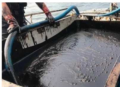
Recovery of floating fuel oil spill from the Makassar Highway in inshore waters: launching an oleophilic skimmer with linear brushes (Lamor Bow Collector) from a recovery barge (left); transfer of the viscous fuel oil stored in the barge's tanks (right) (source: Kustbevakningen)
