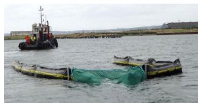
Le *Debris Trawl/River Sweep* (alias le *Scantrawl*) (Source : *DESMI*)
