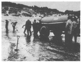
Figure 4. Pumping the oil trapped in a small beach pond by use of a "honey wagon's" vacuum pump
