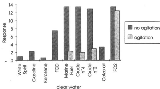
Figure 2. FLUCOMAT response to 33 μL of oil—performance is related to the ratio of surface covered by oil
