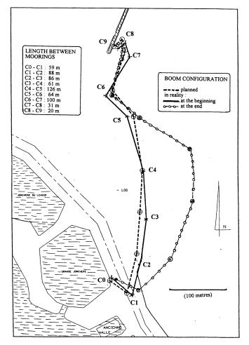
Figure 2. Evolution of the boom configuration
